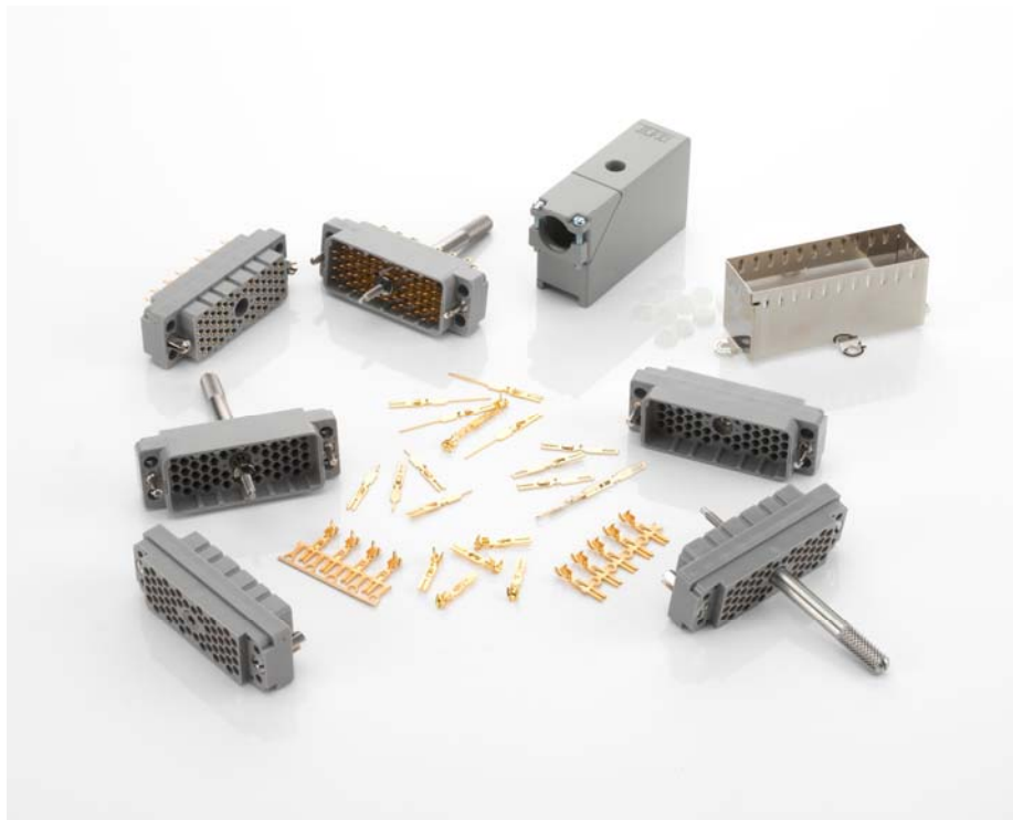
The 56 circuit version of the EDAC 516 connector series showing the EMI/RFI shielding device and metal cover. The plug and receptacle are both shown with either actuating screw or locknut. The hermaphroditic contact is available with crimp; solder eye; pcb or wire wrap tail.
